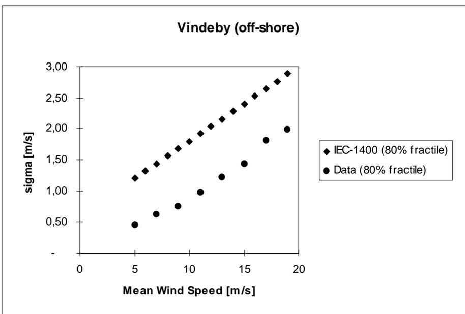
Figure 2.4-5 Standard deviation of horizontal wind turbulence component.
