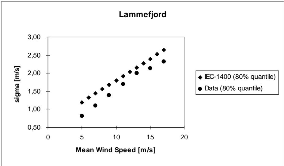
**Figure 2.4-3 Standard deviation of horizontal wind turbulence component.**
