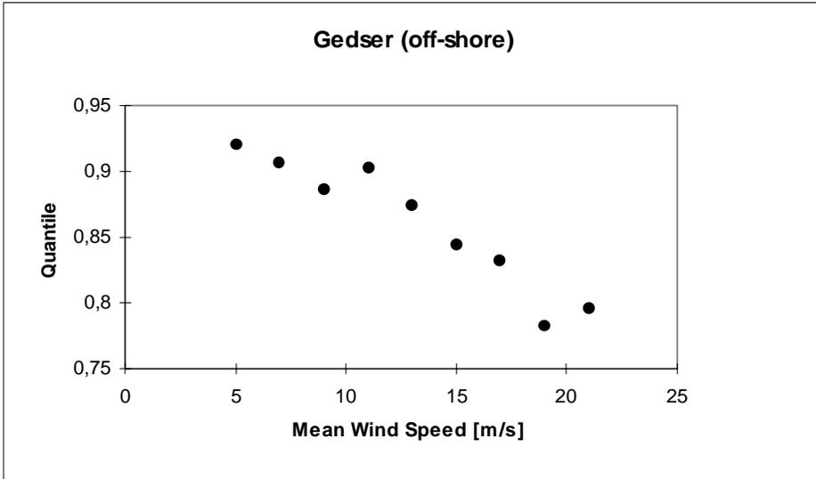
**Figure 2.4-6** Quantiles in the estimated (off-shore) Gedser distributions corresponding to the design standard deviation determined for  $m=12$ .
