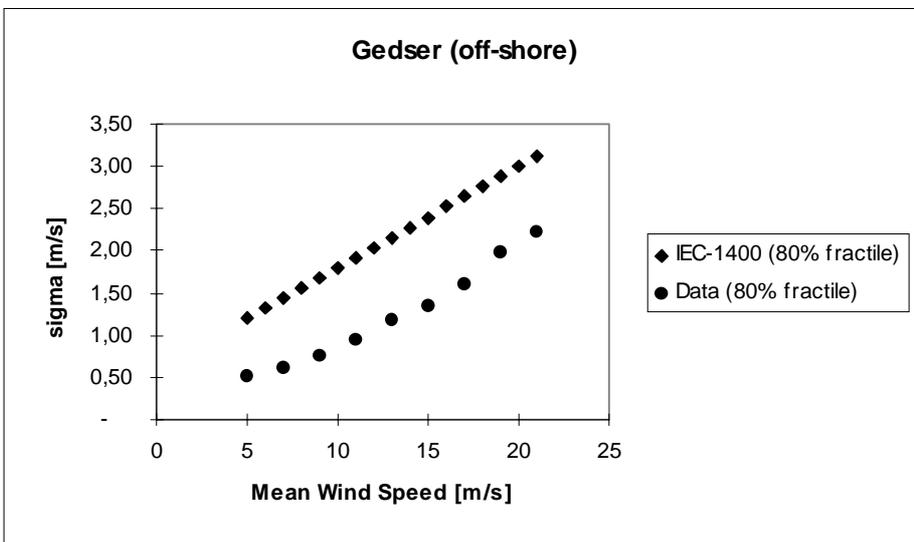
Figure 2.4-4 Standard deviation of horizontal wind turbulence component.
