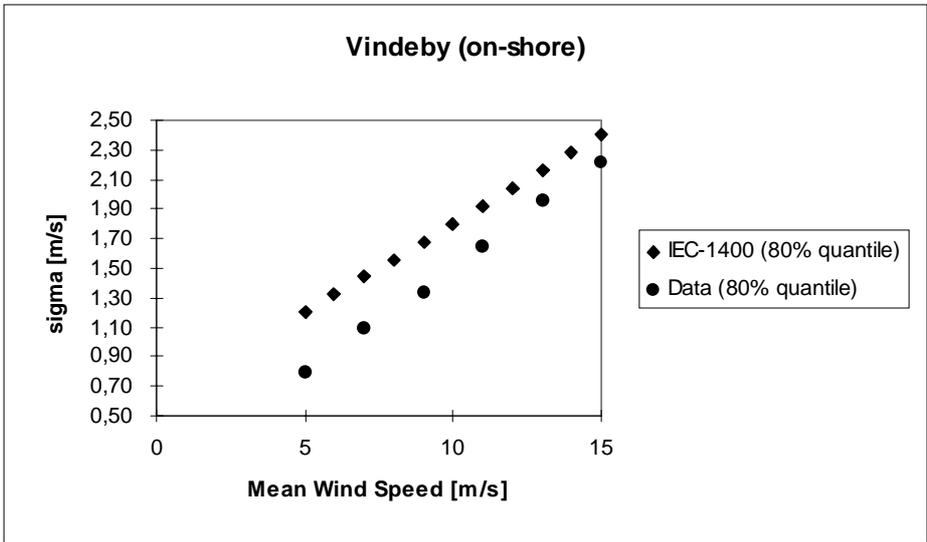
**Figure 2.4-2 Standard deviation of horizontal wind turbulence component.**
