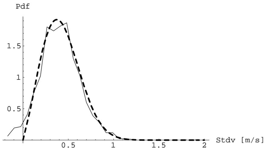
**Figure 2.3-4 Probability density functions representing the mean wind speed bin interval extending from 8m/s to 10m/s. The abscissa values refer to shifted standard deviations.**
