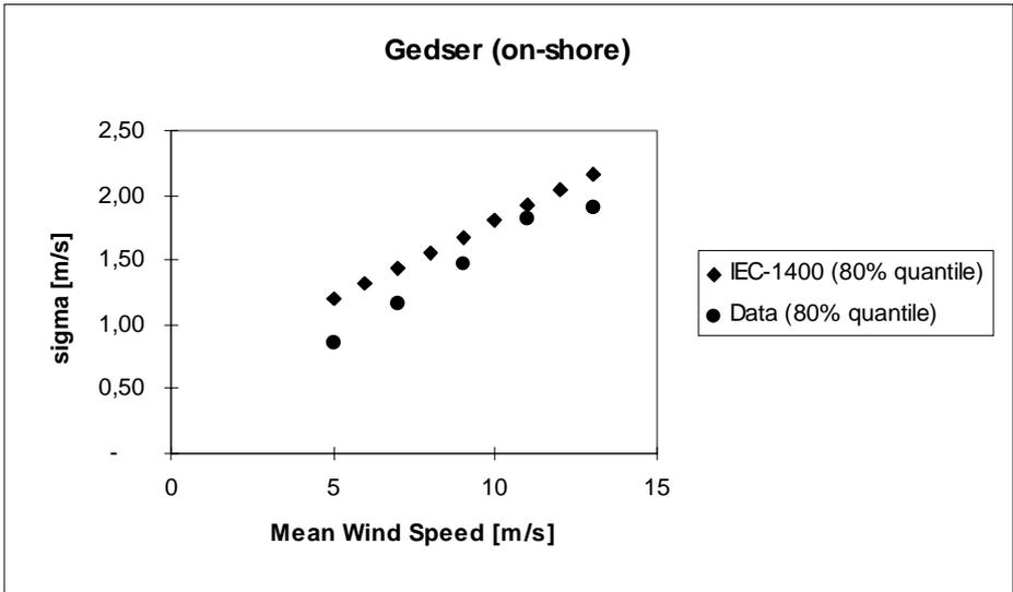
**Figure 2.4-1 Standard deviation of horizontal wind turbulence component.**
