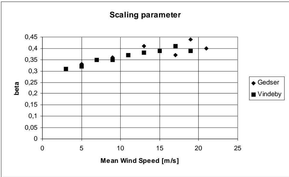
Figure 4-5 Scaling parameter in the Weibull fit associated with off-shore data.
