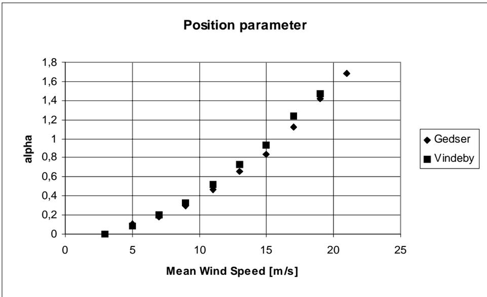
Figure 4-6 Position parameter in the Weibull fit associated with off-shore data.
