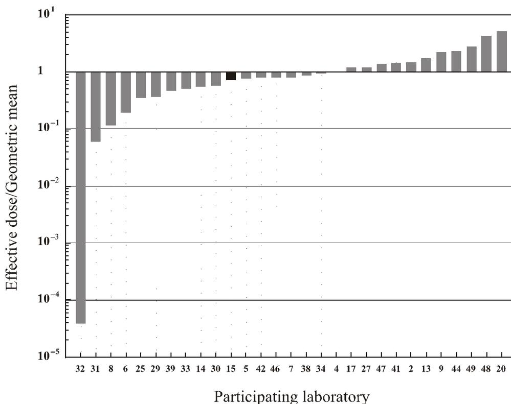
Figure 2.2. Internal dose calculation from intake of  $^{239}\text{Pu}$  with unknown time of intake and way of intake (case 7). Laboratory 32 was not included in the geometric mean.
