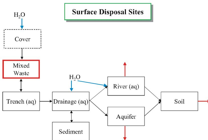
Figure 2.5. Generic compartment scheme for surface disposal sites.
