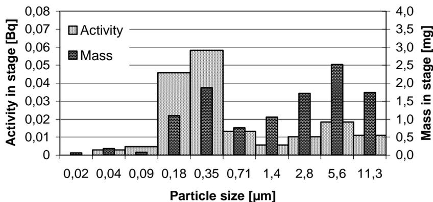
Figure 3.7. Mass and activity distributions from flue gas particles sampled 16 June 1999 at the Rechitza saw mill. The samples were taken after a pilot scale bag house (about 6 m<sup>3</sup> air sample volume) and represent actual release conditions.
