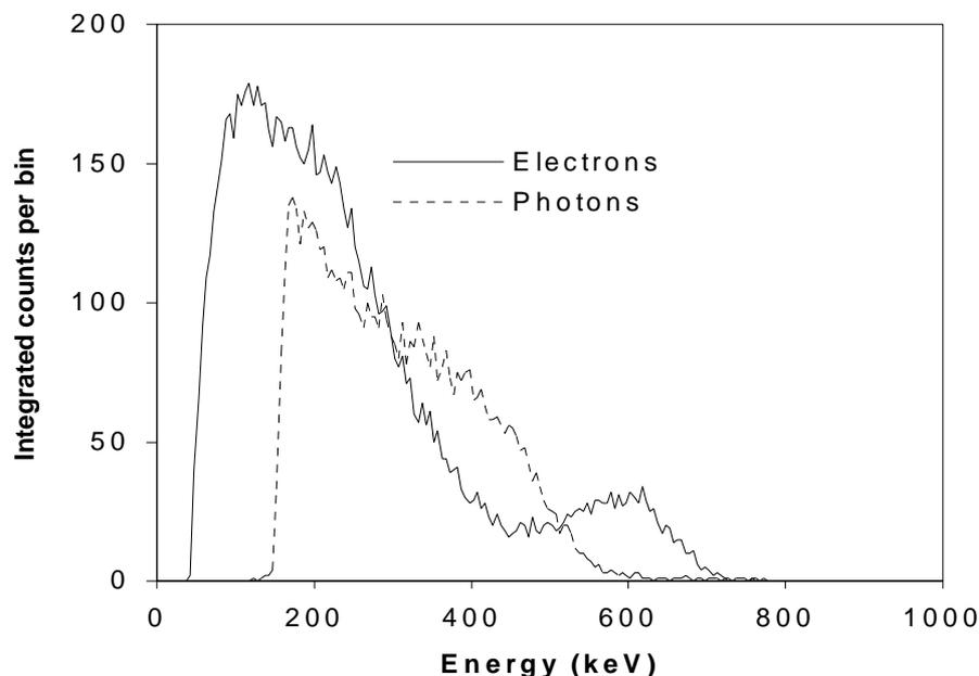
Figure 2.1. Beta and photon spectrum of a 10 mm diameter, 3.7 MBq  $^{137}\text{Cs}$  source covered by a 1 mg/cm<sup>2</sup> Mylar foil measured at a distance of 100 mm by the spectrometer.
