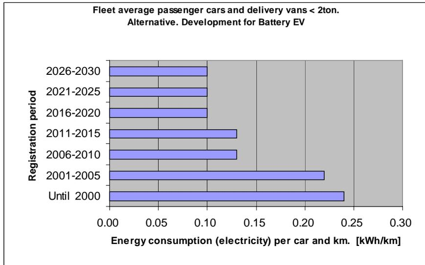
Figure 4-2 Specific energy consumption assumed for future battery electric vehicles (BEV). Passenger cars and delivery vans <2 tons. . Data based on [16]. Units: kWh<sub>el</sub>/km.
