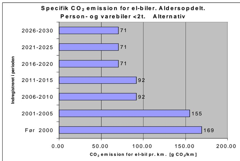
Figure 4-6 Specific CO<sub>2</sub> emissions from battery electric vehicles (BEV). Assumed: Fixed 1997 level electricity supply system CO<sub>2</sub> emission per kWh.
