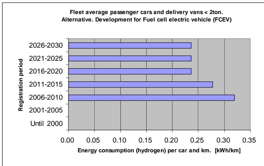
Figure 4-3 Specific energy consumption assumed for future direct hydrogen fuel cell vehicles (HFCV). Passenger cars and delivery vans <2 tons. Data based on [6]. Units: kWh<sub>e</sub>/km.
