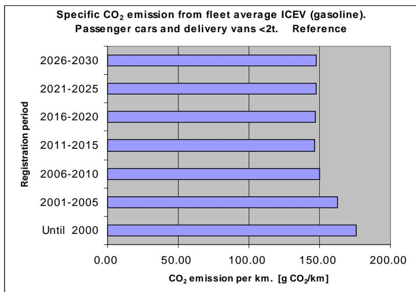
Figure 4-5 Specific CO<sub>2</sub>-emission for passenger cars and delivery vans <2 tons. Based on forecasts of Danish transport work and fleet development from The Road Directorate, Ministry of Transport, Denmark.
