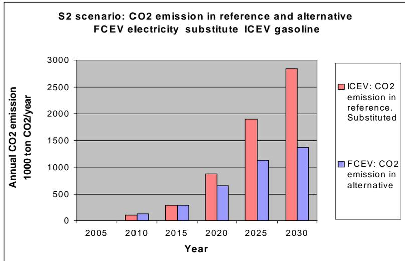
Figure 5-17 CO<sub>2</sub> emissions in scenario S2 and in the baseline development. Electricity production CO<sub>2</sub> characteristics: Development according to the Danish Energy21, The Plan scenario.
