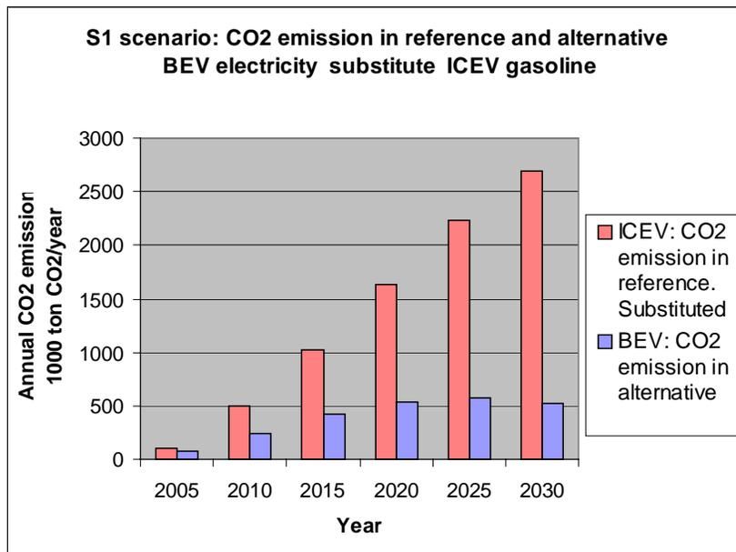
Figure 5-14 CO<sub>2</sub> emissions in scenario S1 and in the baseline development. Electricity production CO<sub>2</sub> characteristics: Development according to the Danish Energy21, The Plan scenario.
