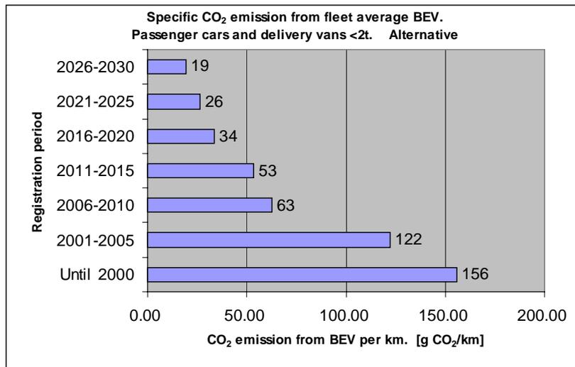
Figure 4-7 Specific CO<sub>2</sub> emissions from battery electric vehicles (BEV). Assumed: Danish electricity supply system development according to Energy21, The Plan scenario [2].
