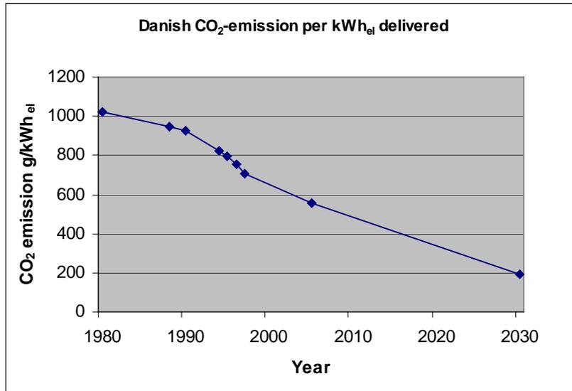
Figure 4-4 CO<sub>2</sub> emission per kWh of electricity delivered at the consumer. Statistics until 1997 from: The Danish Energy Agency. Forecast data beyond year 1997: Based on the Danish energy plan, Energy21, The Plan scenario [2].
