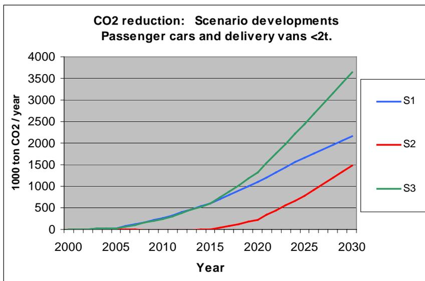
Figure 5-23 CO<sub>2</sub> emission reductions achieved in scenarios S1, S2, S3, relative to the baseline development. Electricity production CO<sub>2</sub> characteristics: Developments according to the Danish Energy21, The Plan scenario.
