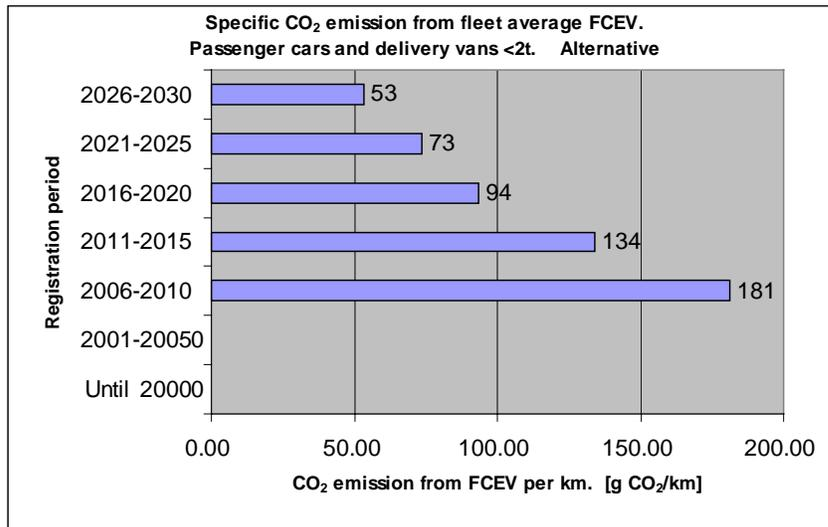
Figure 4-8 Specific CO<sub>2</sub> emissions from direct hydrogen fuel cell vehicles (HFCV). Assumed: Danish electricity supply system development according to Energy21, The Plan scenario [2].
