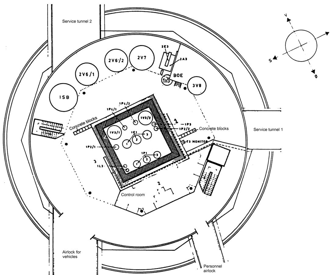
Figure 4 Horizontal cross section, basement level
