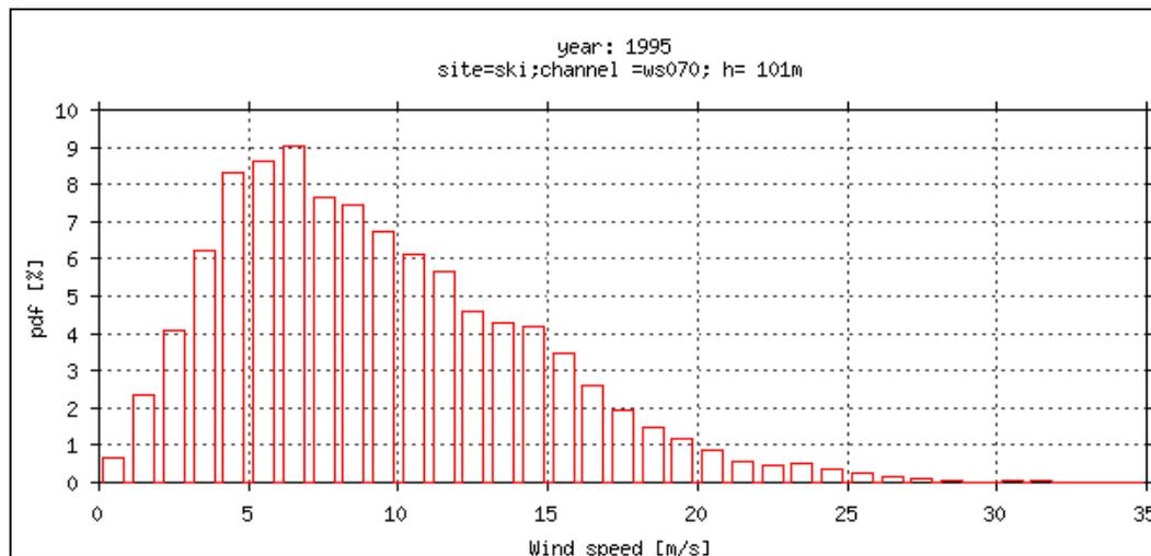
***Distribution of wind speeds, measured at Skipheya, Norway, h=101m, 1995.***
