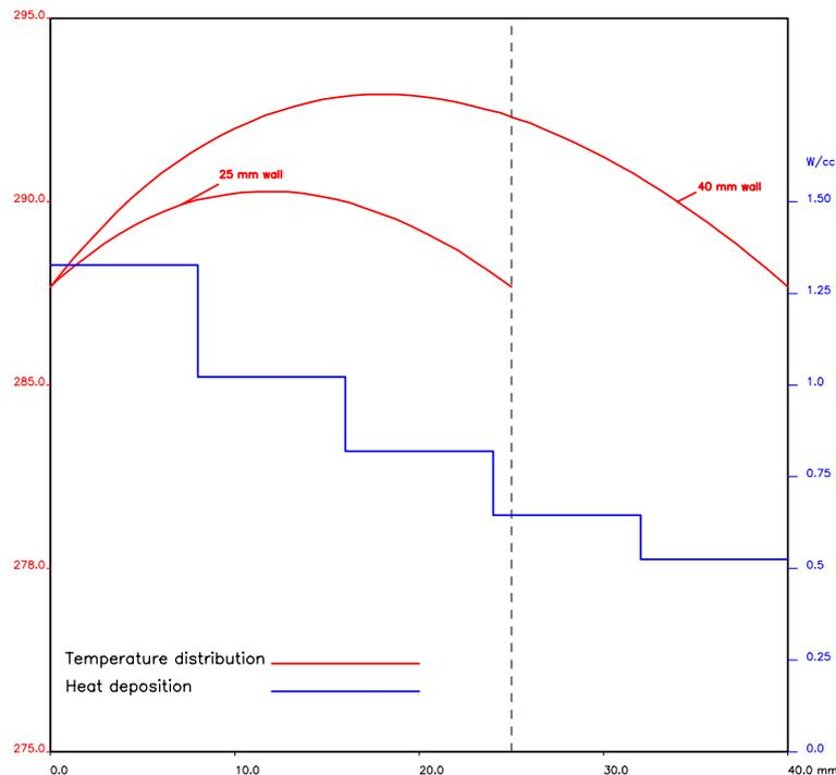
Figure 2.3. The temperature distribution in radial direction in the moderator tank at the core central plane level.
