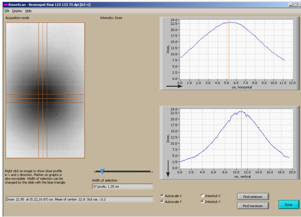
Figure 4.1 RisoeScan measurement of the beam spot at the Risø 10-MeV electron accelerator made with Risø B3 dosimeter film and recorded at a PC-scanner. The dose distribution in the X (horizontal) and Y (vertical) directions are shown.
