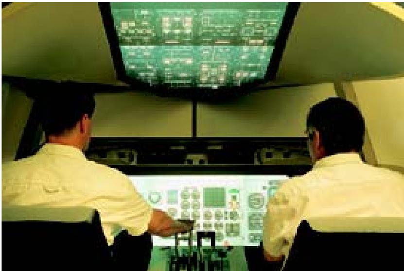
*Figure 3: the MATE cockpit. Touch screens with back projected graphics: the overhead panel and the instrument panel. Real throttles were used in this prototype. Visuals are not a part of MATE because they are not required for procedural training.*
