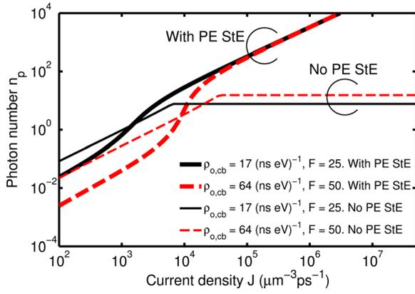
FIG. 3. Light-current characteristics of QD nano-cavity systems with parameters sets  $(\rho_{o,cb} = 17 \text{ (ns eV)}^{-1}, F = 25)$  and  $(\rho_{o,cb} = 64 \text{ (ns eV)}^{-1}, F = 50)$  with and without Purcell enhanced (PE) StE.
