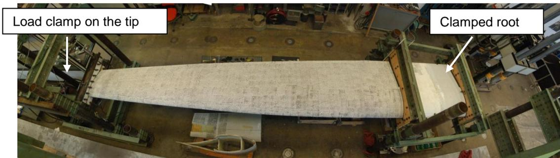
Figure 3. Test rig with the blade section
