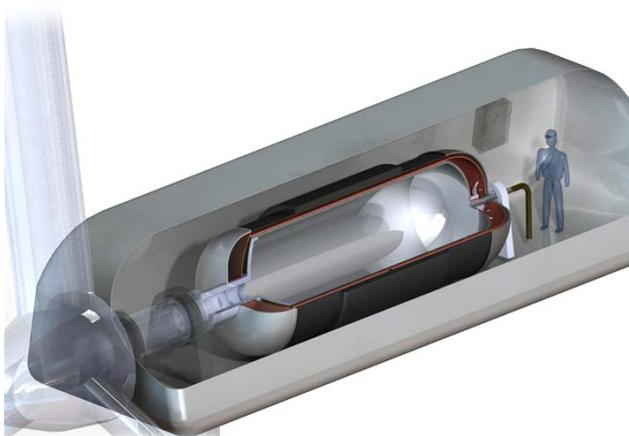
Figure 3 – 10 MW superconducting wind turbine generator with MgB<sub>2</sub> superconductor on both field and armature windings (source: AML)
