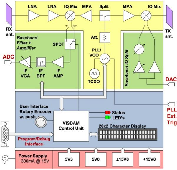
Fig. 2. Block diagram of the DTU-VISDAM radar.
