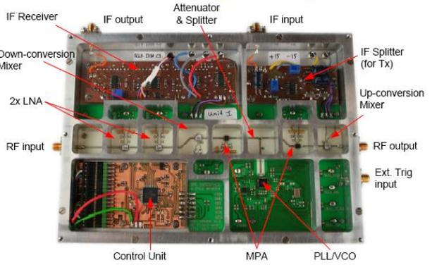
Fig. 4. Photograph of DTU-VISDAM's front-end electronics.
