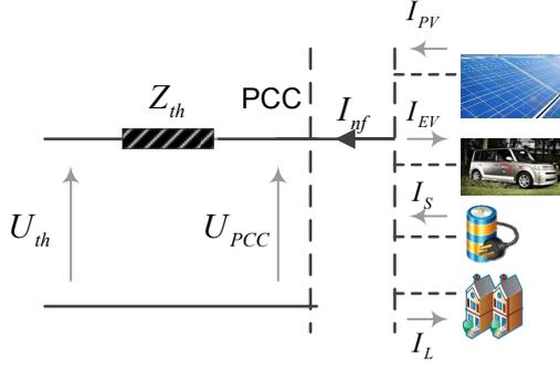
Figure 1. Thevenin equivalent of a typical PV system connected to the grid
