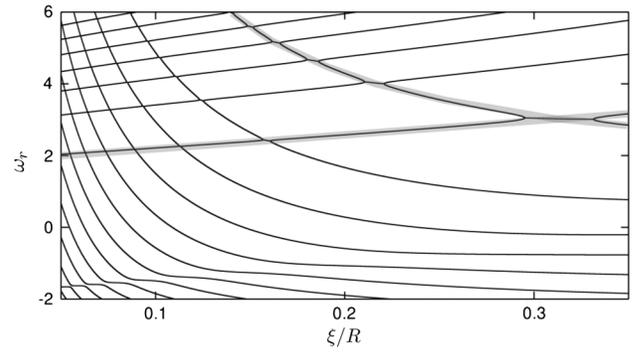
FIG. 3. Oscillation frequencies computed from the full linearized flow (4) and (5) for  $(H/R = 0.276; m = 3)$  as a function of  $\xi/R$ , scaled as in Fig. 2. Only the rightmost instability at  $\xi/R$  slightly above 0.3, the intersection of the shaded lines, is seen experimentally and corresponds to the one in the two-dimensional model at  $\xi/R \approx 0.43$ . The higher resonances are much narrower and weaker.
