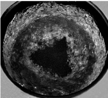
FIG. 5. A rotating triangle formed by stirring liquid nitrogen in a hot kitchen pot. Polygons with  $m = 2, \dots, 6$  are observed during the spin-down process, starting with the  $m = 6$ . The bottom of the pot is Teflon, which gives some unwanted reflections in the dark triangle.
