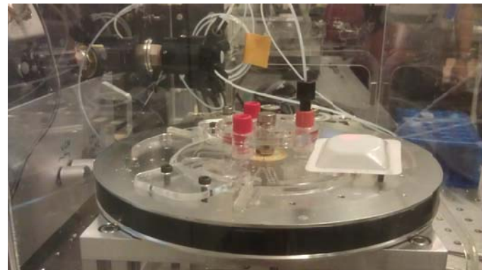
Figure 2: The DVD-ROM optical setup. A PMMA microfluidic disc contains the cantilevers. These are scanned by the DVD-ROM head which detects the deflection of the cantilevers.
