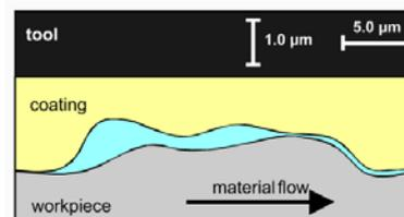
Figure 12. Tool pocket profile and suggested lubrication mechanism [56].
