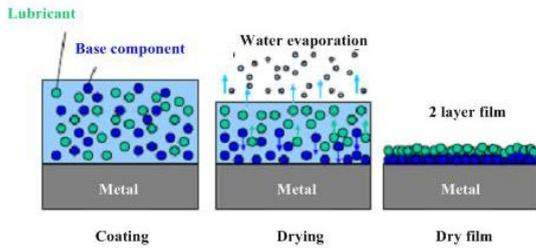
Figure 4. Schematic outline of Dry-in-Place method, PULS [5].
