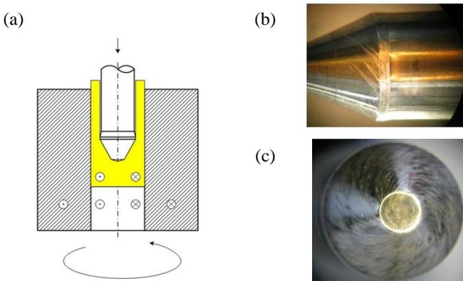
Figure 18. Backward can extrusion twist test [79].
