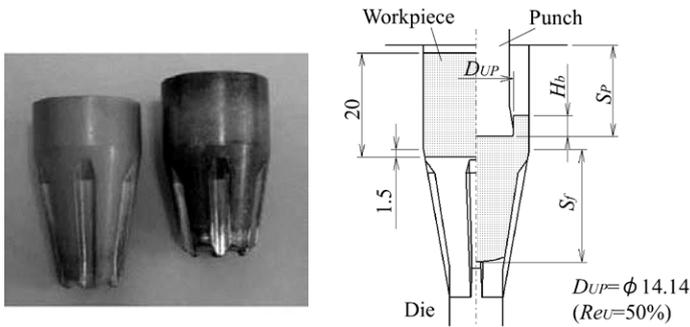
Figure 17. Combined Backward can extrusion twist test [79].
