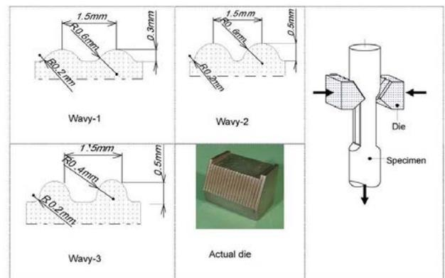
Figure 16. Spike test [75].
