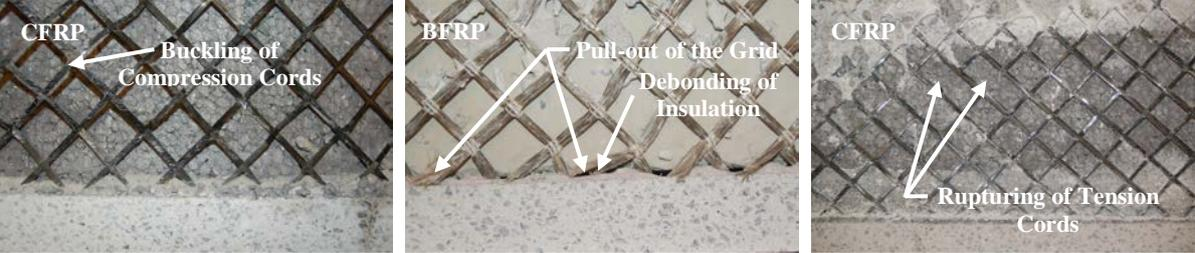
Figure 5. Typical failure modes of push-off test specimens
