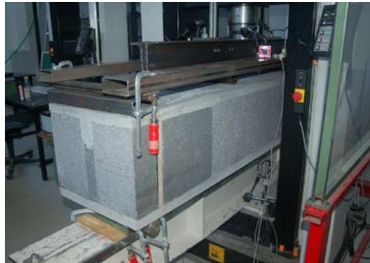
a) Flexural test setup
