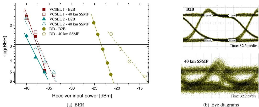
Fig. 2. Measured BER back to back (B2B) and after 40 km SSMF bidirectional transmission. Direct detection (DD) direction, single transmission using VCSEL<sub>1</sub> is included for reference.
