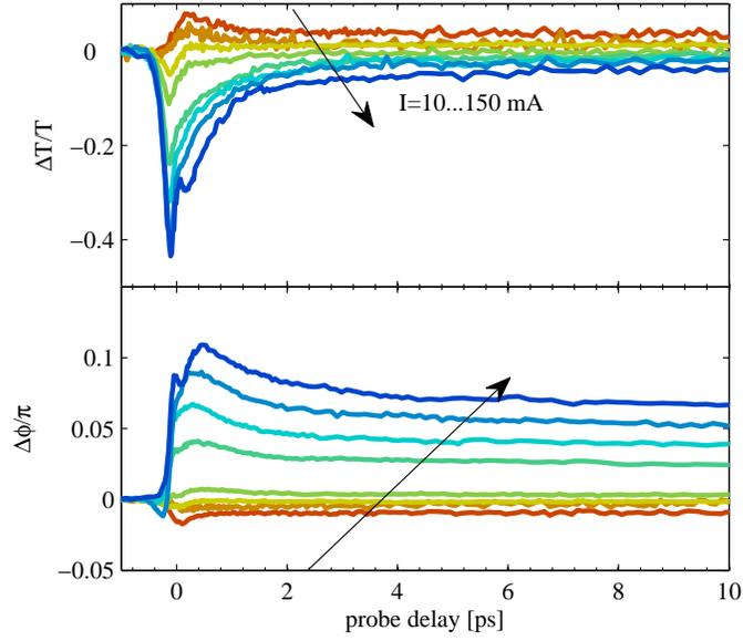
**Figure 2.** (color online) Example of the differential transmission (top) and phase change (bottom) for a weak pump energy carried out at 1525 nm. Applied currents, as indicated by the arrow, are  $0.37I_{tr}$ ,  $0.56I_{tr}$ ,  $0.93I_{tr}$ ,  $1.11I_{tr}$ ,  $1.85I_{tr}$ ,  $2.78I_{tr}$ ,  $3.70I_{tr}$  and  $5.56I_{tr}$  where  $I_{tr} = 27$  mA corresponding to 10...150 mA
