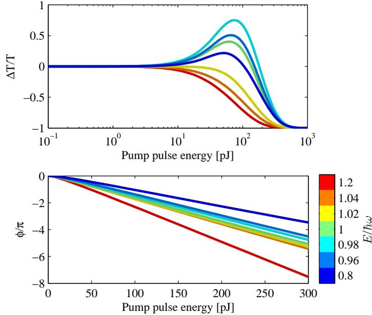
**Figure 6.** (color online) Calculated differential transmission (top) and phase change (bottom) as a function of input pump pulse energy for various photon energies. Photon energies indicated on the legend are normalized to the QDash transition energy of 0.8 eV.
