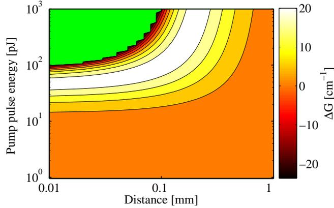
**Figure 8.** (color online) Calculated total modal gain change, i.e.  $\Delta G = \Gamma\Delta g - \Gamma_i\sigma\Delta N$ , as a function of input pump pulse energy and propagation distance at a photon energy of  $1.02E_q$ . For clarity, values below  $-25 \text{ cm}^{-1}$  are not presented in the plot (green color in the upper left corner).
