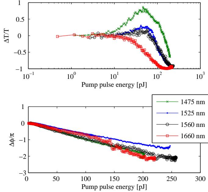
**Figure 4.** (color online) Measured differential transmission (top) and the phase change (bottom) at a probe delay of 7 ps as a function of incoupled pump pulse energy. The measurements series were performed at their respective transparency current apart from 1660 nm that was carried out with no applied current.
