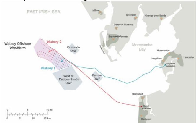
Fig. 1: Walney Offshore Wind Farm 1 + 2 layout and location
