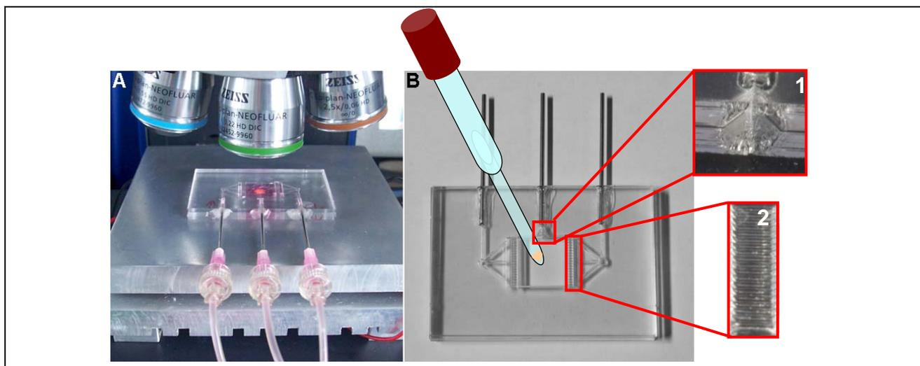
*Figure 1: (A) A single-chamber brain slice culture system designed for culturing on a microscope stage having a Peltier heater. B) A schematic view of tissue loading into the culture chamber and magnification of the chamber design with a funnel-shaped channel (inset 1) and flow equalizers (inset 2).*
