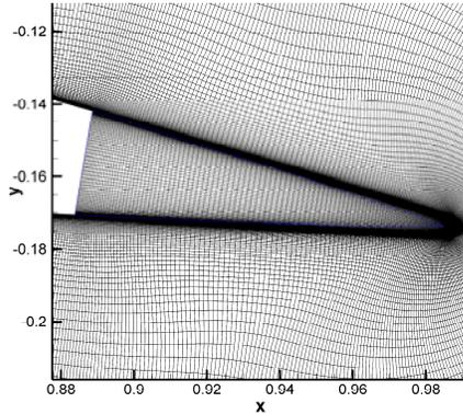
Figure 5. Mesh near the trailing edge part.
