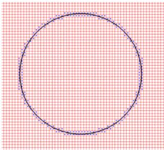
Figure 2. Cartesian mesh for IB simulation.
