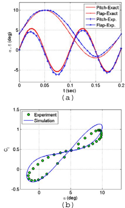
Figure 9. (a) Motion of the pitch and flap angles. (b) Comparison of the computed lift coefficient with experiment at a phase lag of  $148^\circ$ .
