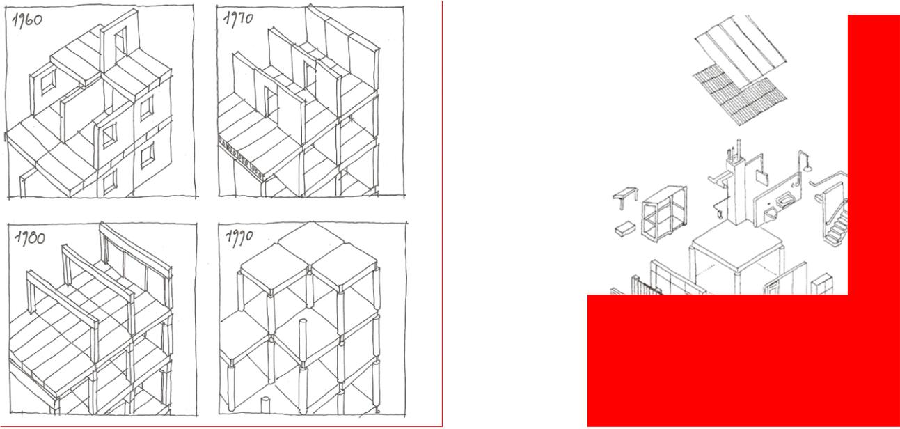
**Figure 3:** The development of the structural systems since the 1960s and the vision for the 1990s (left), showing how the winning project proposes a system consisting of prefabricated components (right).
