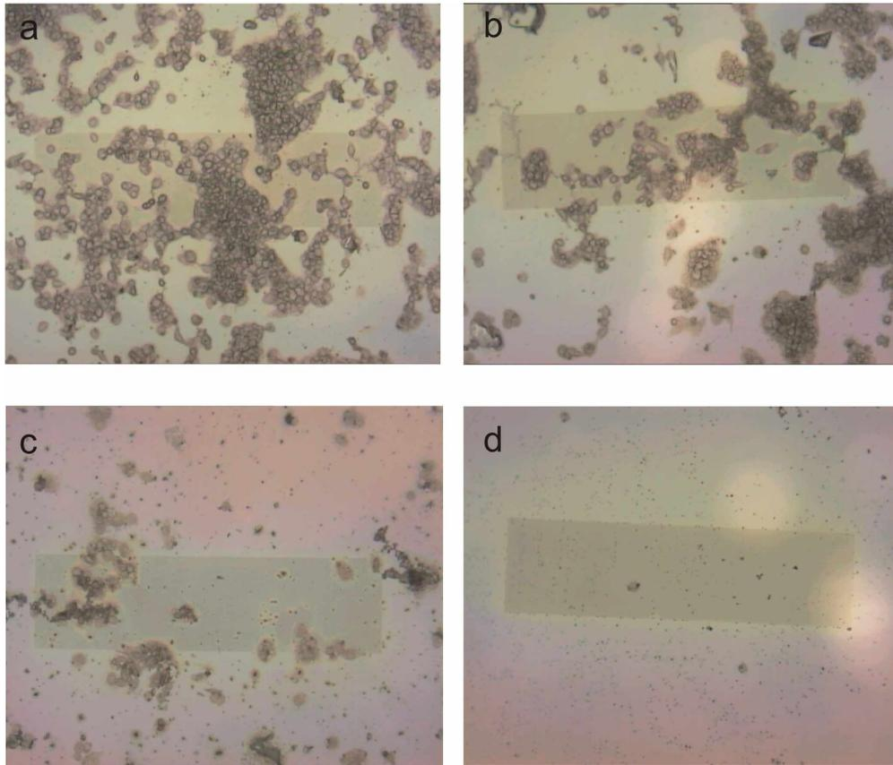
Fig. 3. Laser devices after HeLa cell attachment procedure and drying in air. **(a)** Laser treated with AQ-NH<sub>2</sub> and  $2 \times 10^5$  cells in suspension. **(b)** Laser treated with AQ-NH<sub>2</sub> and  $5 \times 10^4$  cells in suspension. **(c)** Laser treated with AQ-NH<sub>2</sub> and  $1 \times 10^4$  cells in suspension. **(d)** Laser treated with  $2 \times 10^5$  cells in suspension, but no AQ-NH<sub>2</sub>.
