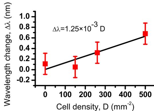
Fig. 4. Measured data and linear fit for the wavelength change in PMS as a function of cell surface density. 500 cells per mm<sup>2</sup> corresponds to a dense film in growth medium, but in PBS the cells contract. Note that the data has been normalized to intercept the origin.
