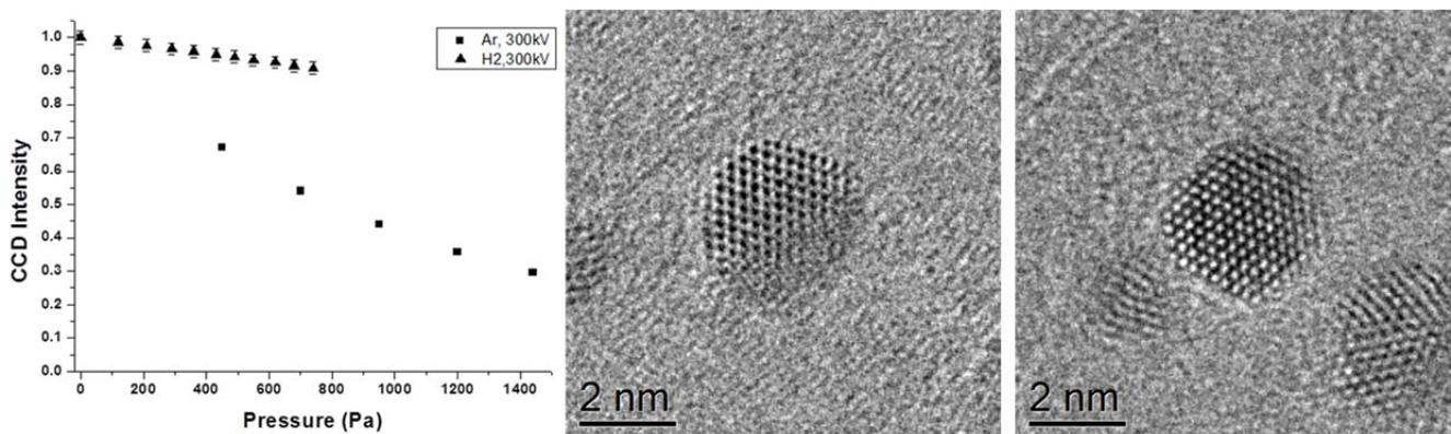
**Figure 1:** Left: Variation in intensity measured on the CCD as a function of gas pressure in the sample region; middle: graphene-supported Au nanoparticle imaged in vacuum; right: Au nanoparticle imaged in hydrogen at 200Pa.
