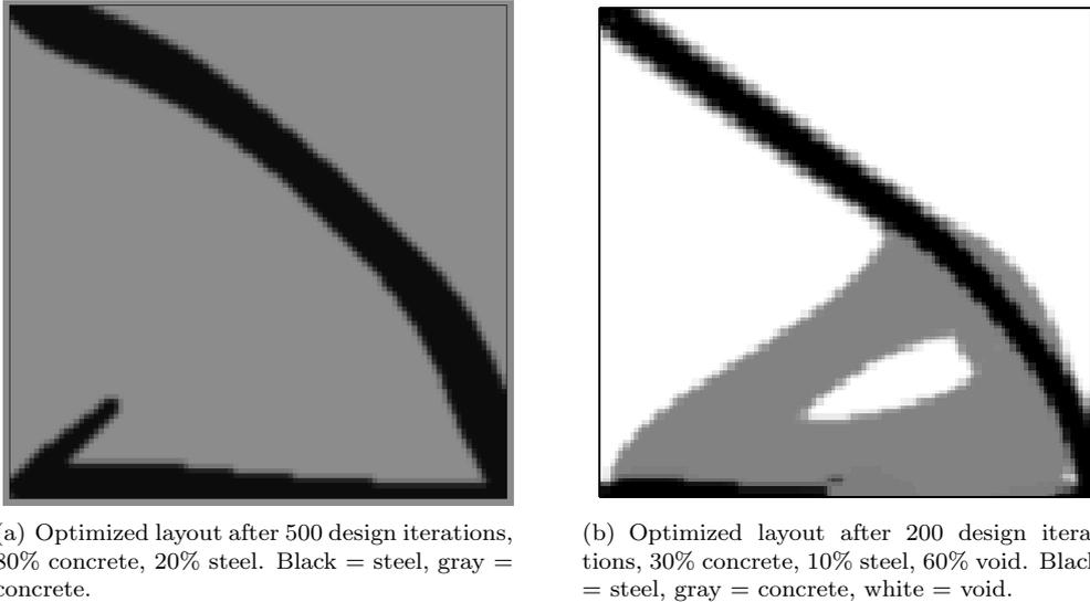
Figure 4: Maximum end-compliance of a short cantilever
