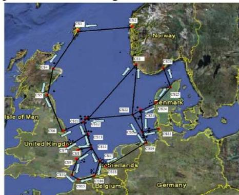
Fig. 1. An example topology of offshore super-grid [14].
