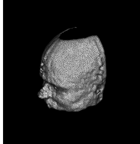
Fig. 4. The output from the TX segmentation. The point cloud was surface reconstructed [13] for the purpose of illustration. Notice that it is possible to see the start of the ear canal, however the ear is missing. Small indentations and bumps are present and the very top and the back-side of the head has been excluded.
