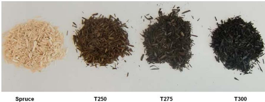
Figure 1. Color change during the torrefaction process.
