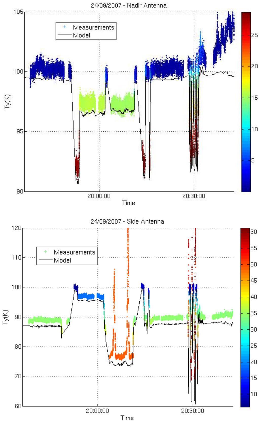
**Figure 9.** Top: Variations in  $T_y$  (1s averages) as observed (colored points), and simulated using the 2scale/DV2 (black) and SSA/Kudr. (grey) models during three circular flights. The azimuth angle is color coded. Bottom: Modeled variations of scattered galactic noise. Left: nadir antenna on 24/09/07; wind speed of 8.3 m/s. Right: side antenna on 28/09/07; wind speed of 8.4 m/s. (a bias has been artificially added to the measurements, to facilitate visual interpretation).
