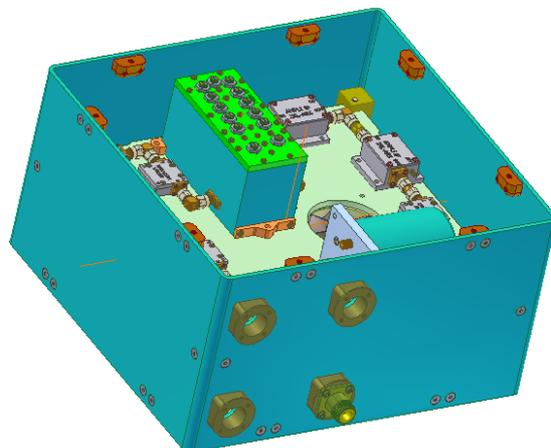
This unit ensures a gain of 81 dB for each channel and an isolation of approximately 80 dB between the H (Horizontal) and V (Vertical) channels. Special attention was paid to the performance of the bandpass filter design. This device, based on cavity properties, provides a center frequency of 1,413 MHz and a 3 dB bandwidth of 24 MHz. The filter was specially tuned to attenuate interfering signals lying outside the bandwidth of interest.
