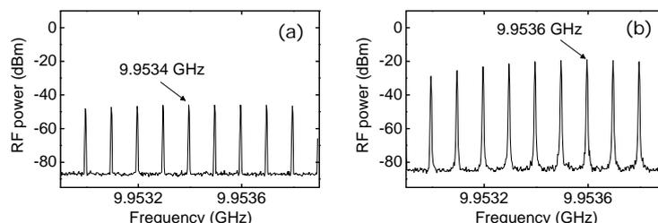
Fig. 3. (a) Electrical power spectrum of the input NRZ packet; (b) the synchronized RZ packet.
