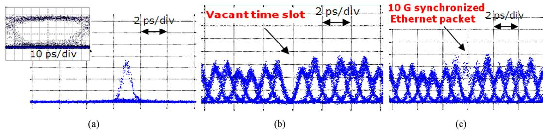
Fig. 4. (a) Optical sampling oscilloscope diagrams of the 10 Gb/s synchronized, retimed and compressed RZ packet ; (b) the 1.28 Tb/s OTDM serial signal with a vacant time slot ; (c) the synchronized Ethernet packet multiplexed with the 1.28 Tb/s signal. Inset: 10 Gb/s input NRZ packet.
