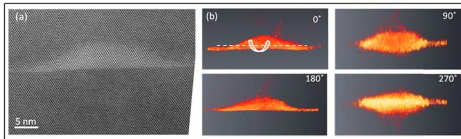
**Figure 3:** (a) HAADF STEM image of a buried InAs/InGaAsP QD viewed along the [110] direction in cross-sectional geometry. (b) Reconstructed image of the same QD from 37 images acquired at  $2^\circ$  intervals over a  $\pm 36^\circ$  tilt range. The reconstruction was carried out using the SIRT algorithm (15 iterations). The arrow indicates the direction of rotation.
