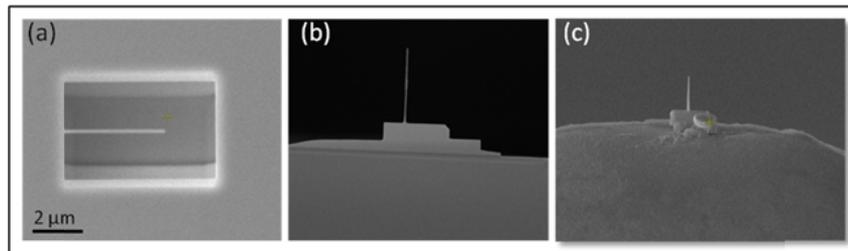
**Figure 5:** (a) Scanning electron microscopy images of needle-shaped specimens fabricated using reactive ion etching, selective wet etching and critical point drying. The needle specimens can be (b) detached from substrates by cleaving or (c) lifted out and mounted onto a suitable grid.
