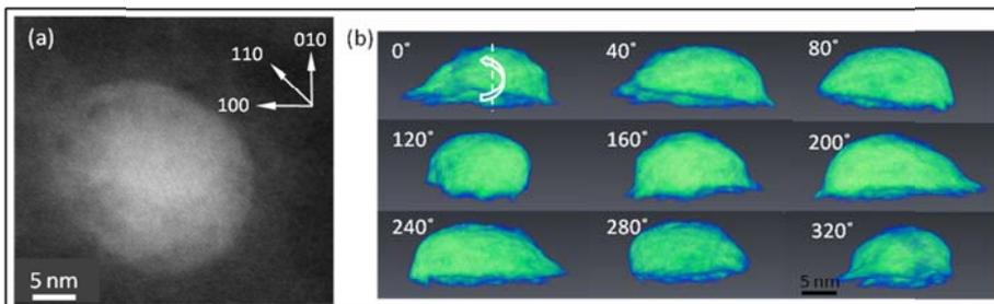
**Figure 4:** (a) HAADF STEM image of a buried InAs/InGaAsP QD in plan-view geometry viewed along the [001] orientation. (b) Tomographic reconstruction of the QD from 61 images acquired at  $2^\circ$  intervals over a  $\pm 60^\circ$  tilt range using the SIRT algorithm (15 iterations). The arrow indicates the direction of rotation.
