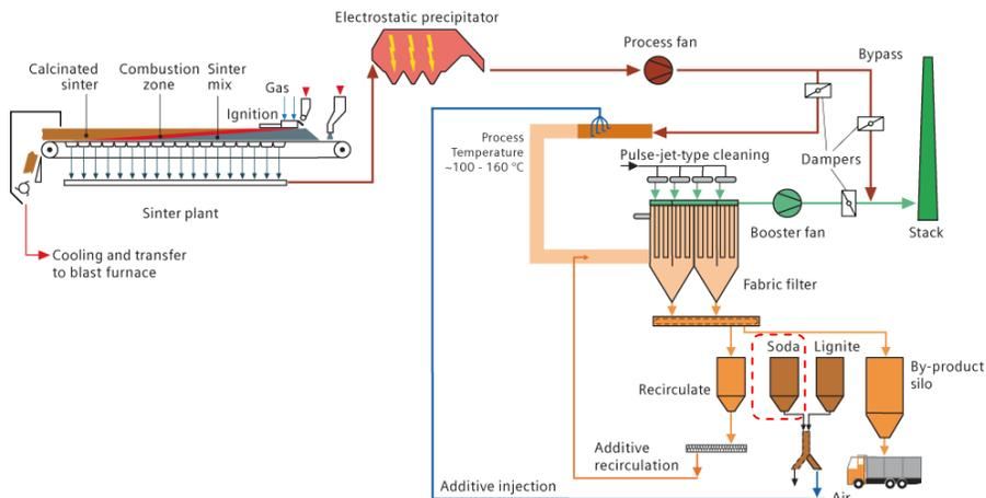
Figure 3b: Process flow sheet of the MEROS<sup>®</sup> plant with NaHCO<sub>3</sub> and lignite as additive
