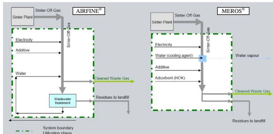
Figure 5: AIRFINE<sup>®</sup> system and MEROS<sup>®</sup> system with system boundaries
