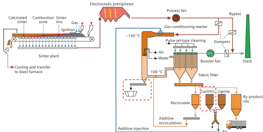
Figure 3a: Process flow sheet of the MEROS<sup>®</sup> plant with Ca(OH)<sub>2</sub> and lignite as additive
