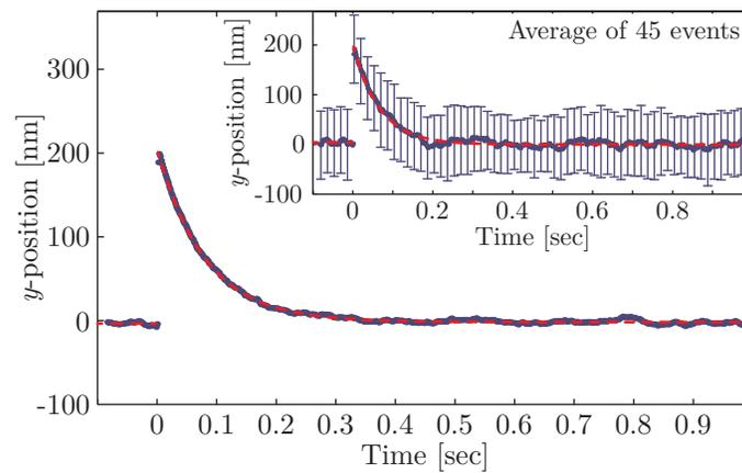
Fig. 3. Plot of the bead's averaged  $y$ -position as a function of time (blue dots). Averaging 450 events like the seven shown in Fig. 2 gave this result. The inset shows the same for the average of 45 events including error bars (shown for every tenth data point), which indicate the standard deviation of the 45 measurements, i. e. the magnitude of the thermal motion. The fits of Eq. (3) are shown by the red dashed lines. They are almost indistinguishable from the data.
