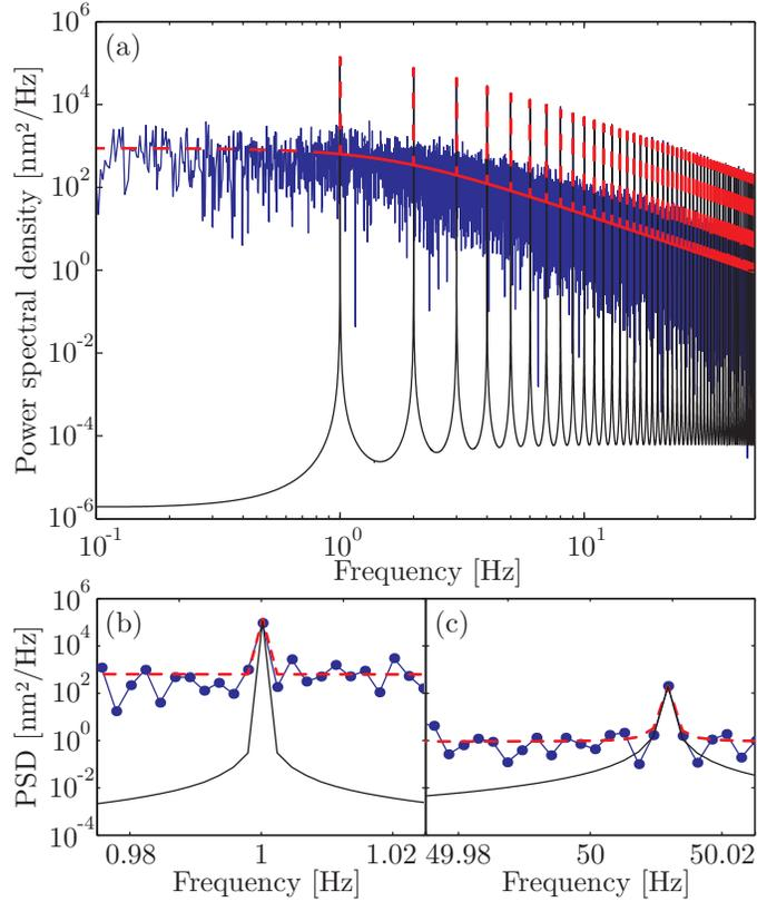
Fig. 5. (a) The measured power spectrum of the bead motion when subject to the laser pulses (blue line). The red dashed line is a fit of Eq. (8). The black line is a plot of the periodic pulsed part of the fit. (b)–(c) Closeup of the peaks at 1 Hz and 50 Hz respectively (connected blue dots). The pulse rate was found to be  $f_p = 1.0002$  Hz.
