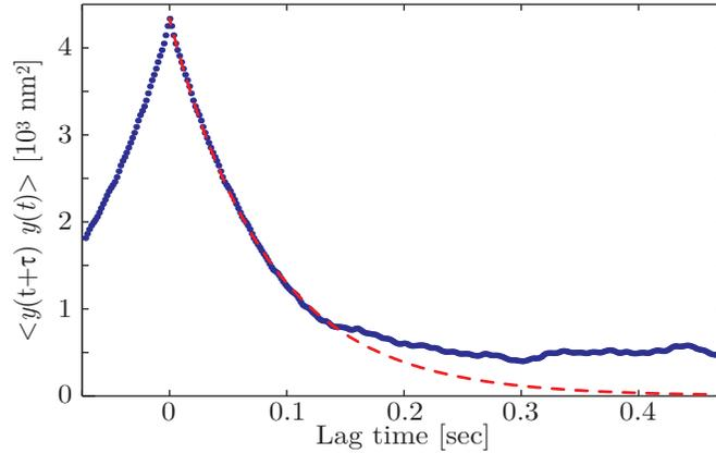
Fig. 4. Example of the position correlation function (dots) of a 17 second long data section without the laser pulses. The fit of Eq. (1) (red dashed line) was performed for  $0 < \tau < 1.2\tau_t = 0.1 \text{ s}$ .
