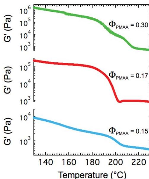
**FIGURE 4** Isochronal temperature sweep measurements of  $G'$  for the systems of S(MD)-MAA(PD)-15 (blue), S(MD)-MAA(PD)-17-M (red), and S(MD)-MAA(PD)-30-M (green) measured at 1% strain amplitude and a frequency of  $\omega = 1 \text{ rad s}^{-1}$ .
