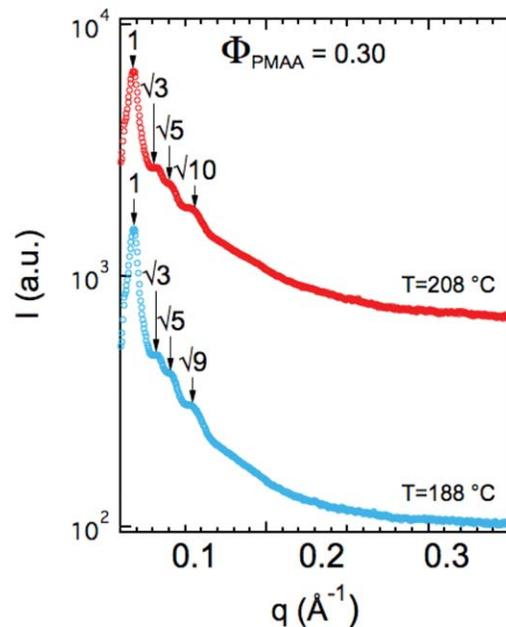
**FIGURE 7** SAXS results for the mixture system of S(MD)-MAA(PD)-30-M at  $T = 188$  °C (blue) and  $T = 208$  °C (red). Observed BCC reflections are identified. All samples were non-birefringent, when viewed between crossed polarizers.
