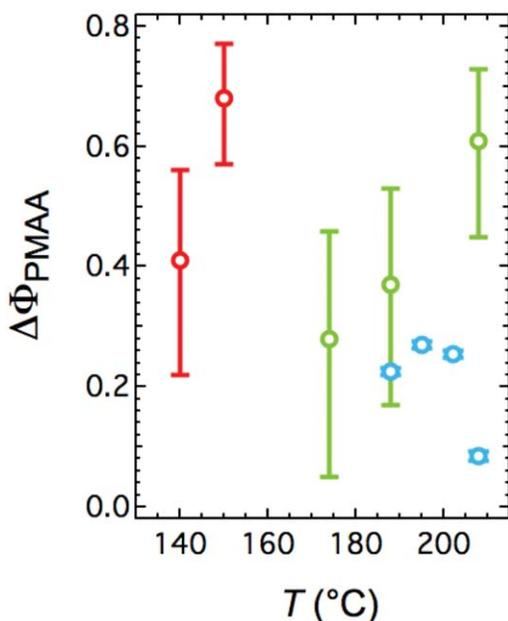
**FIGURE 3** Values of the fraction of the short PMAA blocks  $\Delta\Phi_{\text{PMAA}}$  that are dislodged from the interface and enter into, and swell the PS matrix are shown for different annealing temperatures  $T$  for S(MD)-MAA(PD)-3 (red; using eq 7), S(MD)-MAA(PD)-8-M (green; using eq 7), and S(MD)-MAA(PD)-17-M (blue; using eq 11). The error bars for each data point were calculated using the uncertainty intervals of the input parameters of the used equation.
