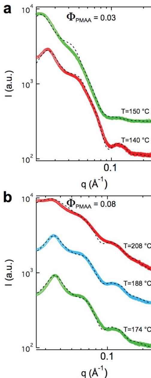
**FIGURE 2** SAXS results for (a) S(MD)-MAA(PD)-3 at  $T = 140$  °C (red) and  $150$  °C (green), and (b) S(MD)-MAA(PD)-8-M at  $T = 174$  °C (green),  $188$  °C (blue), and  $208$  °C (red). In (a) and (b) dashed black lines through the data are the simulated intensities of the proposed model for the SPH microdomains (eqs 2–6).
