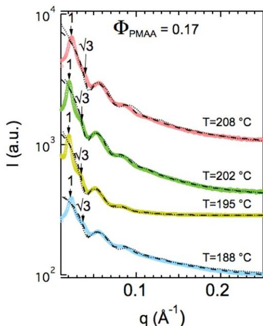
**FIGURE 6** SAXS results for the mixture system of S(MD)-MAA(PD)-17-M at  $T = 208^\circ\text{C}$  (red),  $T = 202^\circ\text{C}$  (green),  $T = 195^\circ\text{C}$  (yellow), and  $T = 188^\circ\text{C}$  (blue). The first two reflections of BCC are specified. The dashed and the dotted lines are the results of simulation to the sphere and cylinder form factors, respectively (see Table 3 for the simulation parameters). The samples were not birefringent when viewed between crossed polarizers.
