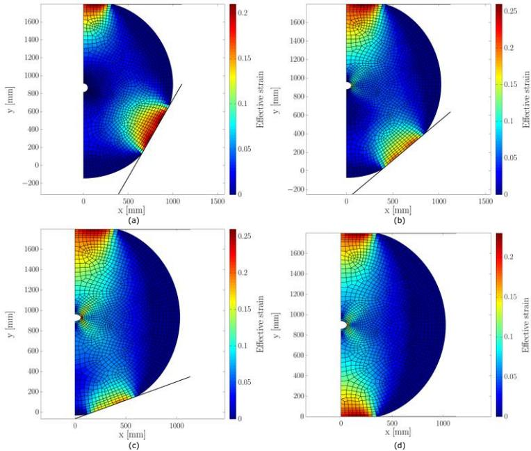
Fig. 5. Effective plastic strain when forging an ingot having a flow stress  $\sigma_0 = 100MPa\left(\frac{\dot{\epsilon}^{pl}}{\epsilon}\right)^{0.4}$  using lower die angles of  $60^\circ$  (a), of  $100^\circ$  (b), of  $140^\circ$  (c) and  $180^\circ$  (d).
