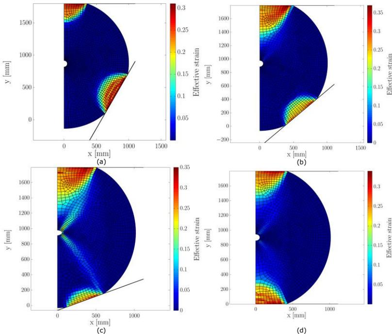
Fig. 3. Effective plastic strain when forging an ingot with constant flow stress,  $\sigma_0 = 100$  MPa using lower die angles of  $60^\circ$  (a), of  $100^\circ$  (b), of  $140^\circ$  (c) and  $180^\circ$  (d).
