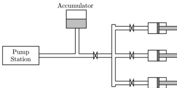
Figure 9. The hydraulic pitch system with three actuators.
