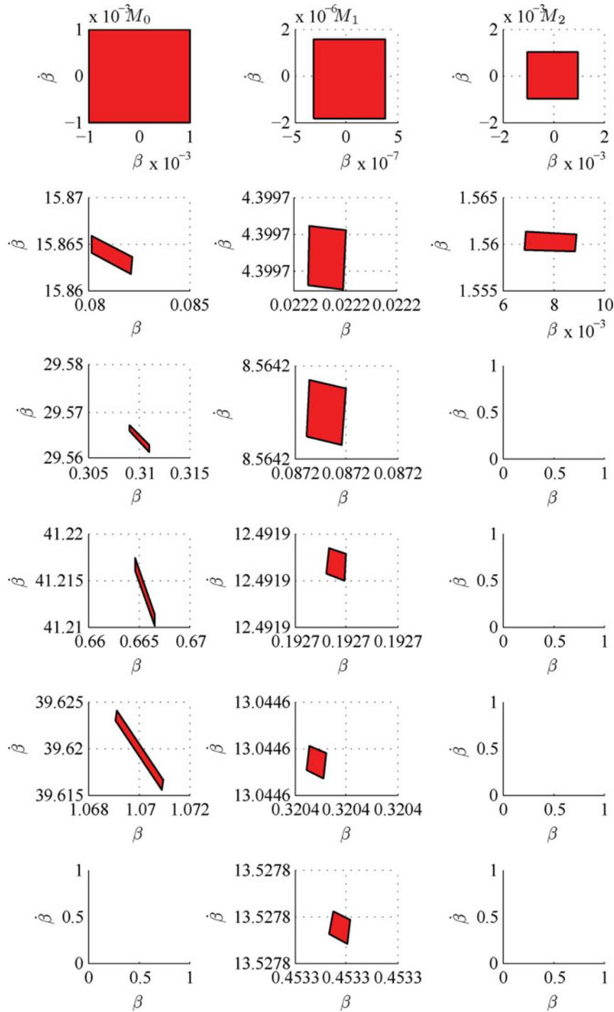
Figure 12. Evolution of  $\mathcal{X}_i^c(k)$  for the pitch system in different conditions over time. Columns show the system in different conditions: nominal system  $M_0$ , the system subject to the pressure drop fault  $M_1$ , and subject to air content increase  $M_2$ . Each row represents a sample time.
