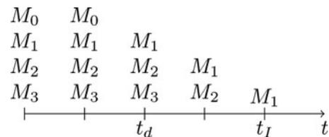
Figure 2. Example of fault detection and isolation using model falsification; each column shows the un-falsified models,  $t_d$ : detection time,  $t_I$ : isolation time.
