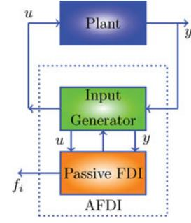
Figure 4. General structure of an AFDI module.
