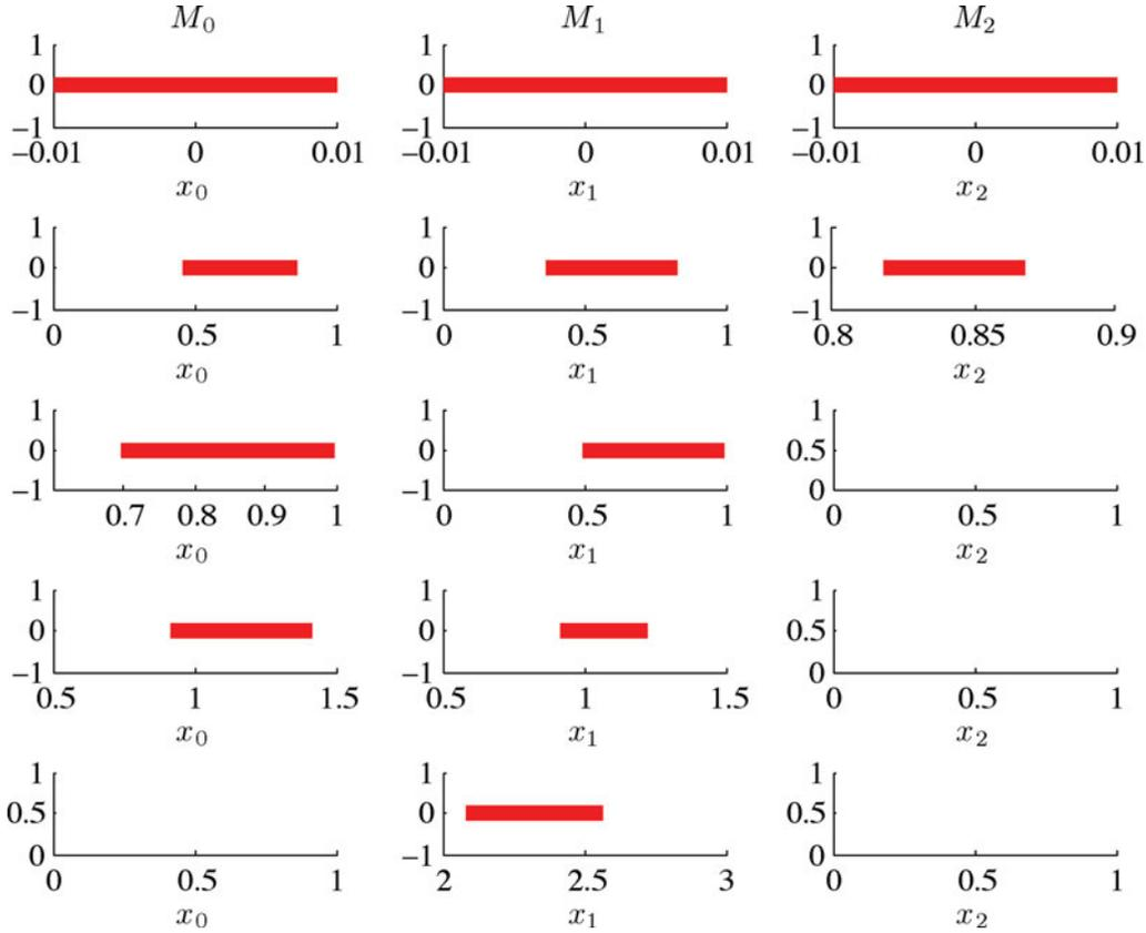
Figure 6. Evolution of  $\mathcal{X}^c(k)$  for example 1 in different conditions over time. Columns show the system in different conditions: nominal system  $M_0$ , system subject to the pressure drop fault  $M_1$ , and subject to air content increase  $M_2$ . Each row represents a sample time.
