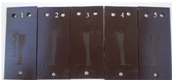
Fig.9 – Surface erosion in PUR rubber material after the tracking resistance tests. Sample 1 failed.
