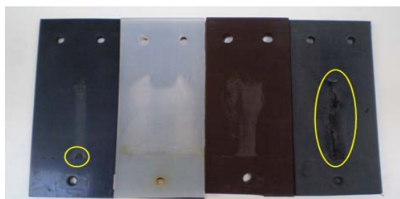
Fig.11 –The surface erosion (marked in yellow) and dry band can be compared in failed samples of each material. From left to right: Santoprene, Silicone rubber, PUR, EPDM.
