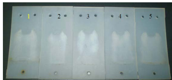
Fig.8 – Surface erosion in Silicone rubber material after the tracking resistance tests. Sample 1 failed.
