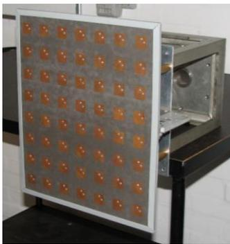
Figure 12 – The 7 by 8 patch array.
