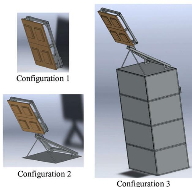
**Fig. 2** BIOMASS feed measurement configurations. Configuration 1 consists of the  $2 \times 2$  patch array and the test support structure. Configuration 2 further includes the triangular support structure and the satellite top plate. Configuration 3 further includes the rest of the satellite structure
