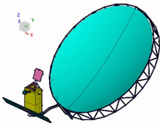
**Fig. 1** One of the possible BIOMASS satellite configurations with the deployable reflector antenna (courtesy of Thales Alenia Space, Italy). The large deployed reflector (blue) is illuminated by the square feed antenna (purple) sitting on its triangular support structure (brown) on top of the box-shaped satellite (green) holding also a deployed rectangular solar panel (brown)
