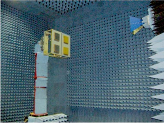
**Fig. 6** Measurement of the feed array (Conf. 1) at the Naval Maintenance Establishment (with permission from [9])
