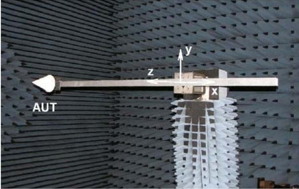
Figure 1. Offset log-periodic antenna used as AUT.
