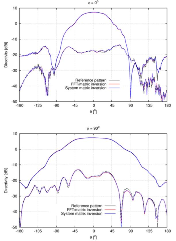
Figure 4. Comparison of the AUT radiation pattern obtained with two high-order probe correction techniques versus reference pattern:  $\phi = 0^\circ$  plane (top) and  $\phi = 90^\circ$  plane (bottom).
