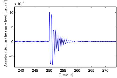
**FIGURE 4:** Acceleration in the pinion of the due to the loss of electromagnetic torque. The wind is constant at 14 m/s.
