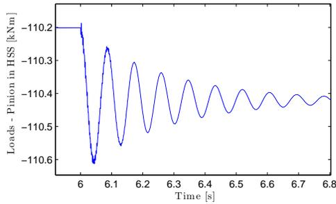
**FIGURE 8:** Torsional loads in the pinion of the HSS due to a change in rotational speed
