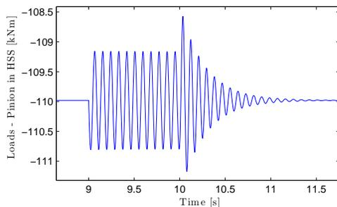
**FIGURE 9:** Torsional loads in the pinion of the HSS due to a loss of the electromagnetic torque in the generator
