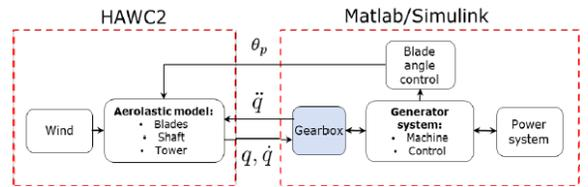
**FIGURE 5:** Wind turbine block diagram (modified from [2])
