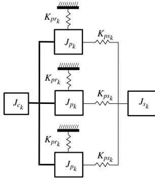
FIGURE 6: Torsional model of a planetary gearbox
