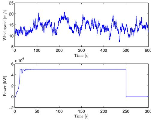
**FIGURE 2:** Simulation cases. *Top:* turbulent wind. *Bottom:* generator power at a steady wind of 14 m/s, with electrical fault at 250 s.
