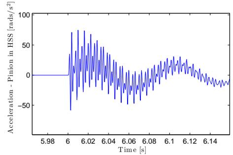
FIGURE 7: Acceleration in the pinion of the HSS due to a change in rotational speed
