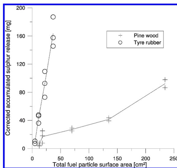
**Figure 9.** Corrected accumulated sulfur release versus the total surface area of pine wood and tire rubber fuel particles. Conditions: 900 °C, 10 vol % O<sub>2</sub>, 5% fill degree, 6 rpm, 100 NL/min.
