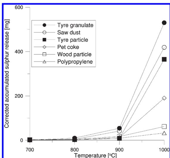
**Figure 7.** Corrected accumulated sulfur release from raw materials as a function of temperature and fuel particle size. Conditions: 5% fill degree, 10 vol % O<sub>2</sub>, 100 NL/min, 6 rpm. Energy input in each experiment: 30 kJ. Sulfur release for tire granulate and sawdust at 1000 °C has been estimated because the SO<sub>2</sub> concentration exceeded the analyzer range for these two specific experiments.
