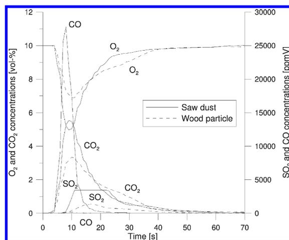
**Figure 8.** Flue gas composition during combustion of a pine wood particle with dimensions 30 × 15 × 10 mm and pine wood sawdust with particle size <1 mm. Conditions: 10 vol % O<sub>2</sub>, 5% fill degree, 1000 °C, 100 NL/min, 6 rpm.
