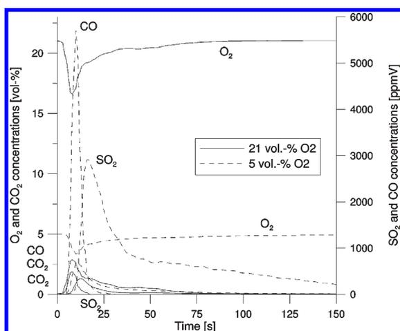
**Figure 11.** Flue gas composition during combustion of 0.81 g (30 kJ) of tire rubber granulate at 5 and 21 vol % O<sub>2</sub>. Conditions: 5% fill degree, 900 °C, 100 NL/min, 6 rpm.
