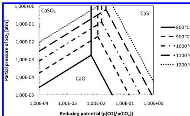
Figure 2. Phase diagram for the  $\text{SO}_2$ – $\text{CaO}$ – $\text{CaSO}_4$ – $\text{CaS}$ – $\text{CO}$ – $\text{CO}_2$  system (based on thermochemical data from Barin).<sup>12</sup>
