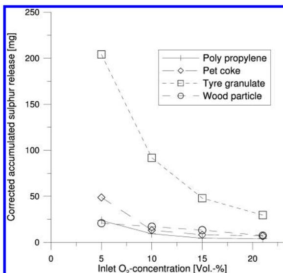
**Figure 10.** Corrected accumulated sulfur release as a function of inlet oxygen concentration for four different fuels. Conditions: 5% fill degree, 900 °C, 100 NL/min, 6 rpm. Energy input in each experiment was 30 kJ.
