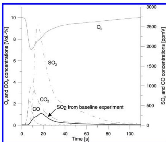
**Figure 5.** Concentrations of  $O_2$ ,  $CO_2$ ,  $CO$ , and  $SO_2$  during an experiment with 0.81 g of tire rubber granulate corresponding to an energy input of 30 kJ. Conditions: 900 °C, 5% fill, 6 rpm, 100 NL/min, 10%  $O_2$ .
