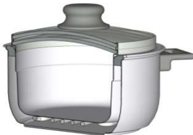
Figure 1. Section view of EffiCooker
