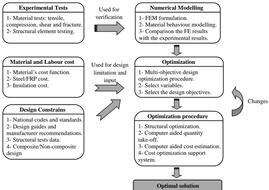
Figure 1. Proposed design optimization methodology of HPCSPs.
