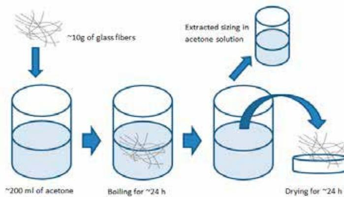
Fig. 2: A schematic presentation of the extraction process.
