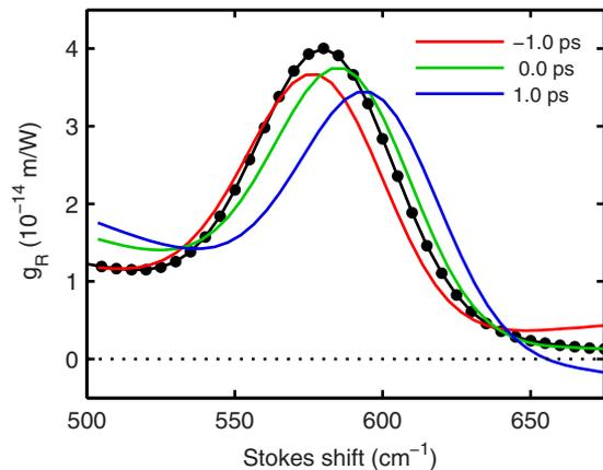
Fig. 5. Raman gain retrieved from the simulations and the Raman gain spectrum input into the simulation (black curve) for zero delay and for a delay of  $-1$  and  $1$  ps. The pump peak power for this simulation is  $500$  W.
