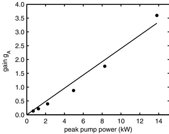
Fig. 3. Stimulated Raman gain as a function of the peak pump power. The points represent the experimentally measured values for a Stokes shift of  $580\text{ cm}^{-1}$ . The full line is a linear fit. The slope of the curve corresponds to a material gain of  $g_R = 4.0 \times 10^{-14}\text{ m W}^{-1}$ .
