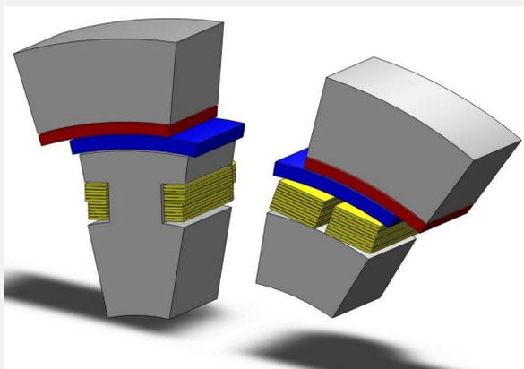
Fig. 1 Conceptual design of one pole section for salient (left) and non-salient (right) synchronous machine with air-gap winding. The magnetic steel is gray, armature winding is dark red, thermal insulation (vacuum chamber, spacers, radiation shields) is blue and space for HTS coils is denoted with yellow.
