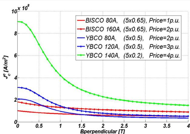
Fig. 2. Estimated engineering current density for 1G and 2G coils at 20 K. Legend reads the HTS type,  $I_c@77K$  in self field, estimated dimensions of cross section of insulated HTS tapes in [mm] and estimated price of the tapes, all normalized to the price of 1G-80A (BISCO-80A). The insulation of the tapes is assumed to be 0.3 mm for glass fiber and 0.15 mm for coated insulation.
