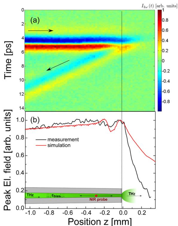
FIG. 3. (Color online) (a) 2D map of THz induced second harmonic  $I_{2\omega}(t)$  as a function of THz wave-probe delay time for different positions of the probe beam along the waveguide. Values of  $I_{2\omega}(t)$  have been corrected for the bias field. (b) Measured and simulated integrated peak THz electric field across the waveguide as a function of NIR probe position  $z$ .
