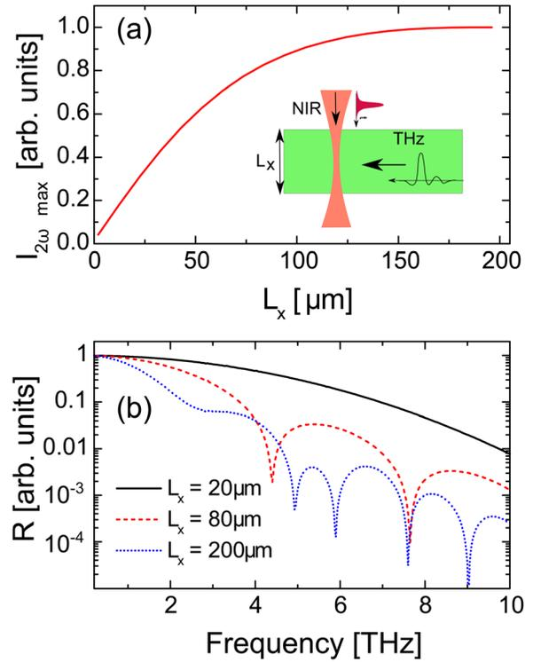
FIG. 2. (Color online) (a) Normalized maximum second harmonic intensity  $I_{2\omega}$  as a function of interaction length  $L_x$  between fundamental and THz beams. The 800 nm beam waist at the focus point has been calculated to be  $6.5 \mu\text{m}$  and the Rayleigh range is  $41 \mu\text{m}$ , pulse duration 90 fs. Inset presents considered geometry. (b) Normalized response function  $R(f)$  for  $L_x = 20 \mu\text{m}$ ,  $80 \mu\text{m}$ , and  $200 \mu\text{m}$ .
