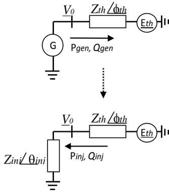
Figure 1. Equivalent system representation regarding critical generator.
