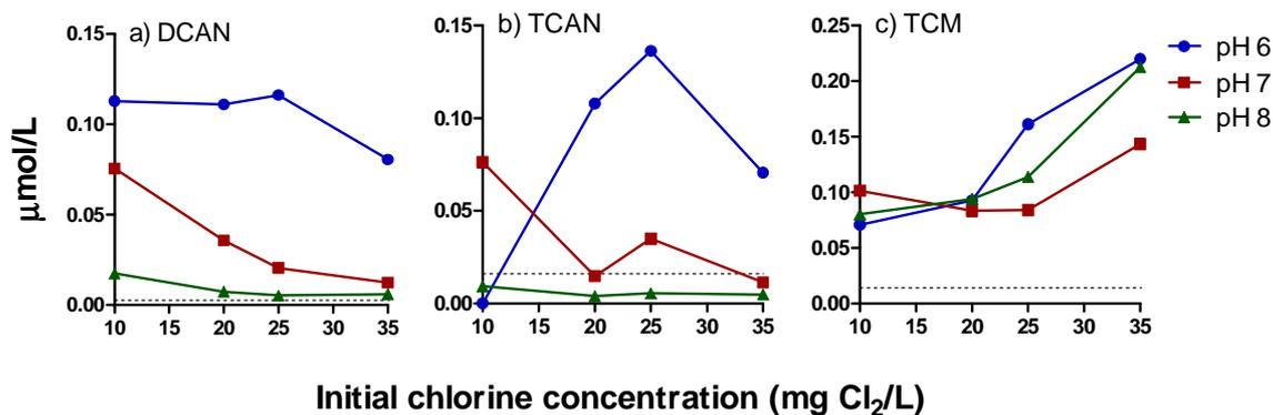
**Figure 1.** Effect of initial chlorine concentration and pH on THM and HAN formation from chlorination of BFA. (Reaction time = 48 h, temperature = 25 °C and BFA addition = 1 mg TOC/L). The dashed line indicates the limit of quantification of the analysis. Abbreviation of compounds is found in Table 1.
