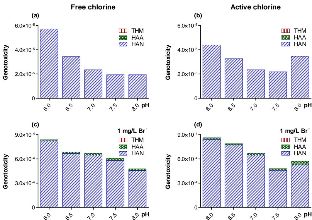
**Figure 6.** Estimated genotoxicity of chlorinated BFA solution with constant initial concentration of free (a,c) and active chlorine (b, d), at  $6.0 \leq \text{pH} \leq 8.0$  in the presence and absence of 1 mg/L Br<sup>-</sup>.
