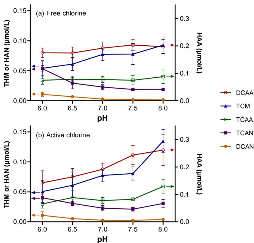
**Figure 2.** Effect of pH on THM, HAN and HAA formation from chlorination of BFA with constant initial concentration of free chlorine (a) and active chlorine (b), in the absence of bromide. The error bars represent the standard deviation of six replicates. (Reaction time = 48 h, temperature = 25 °C and BFA addition = 1 mg TOC/L). Abbreviation of compounds is found in Table 1.
