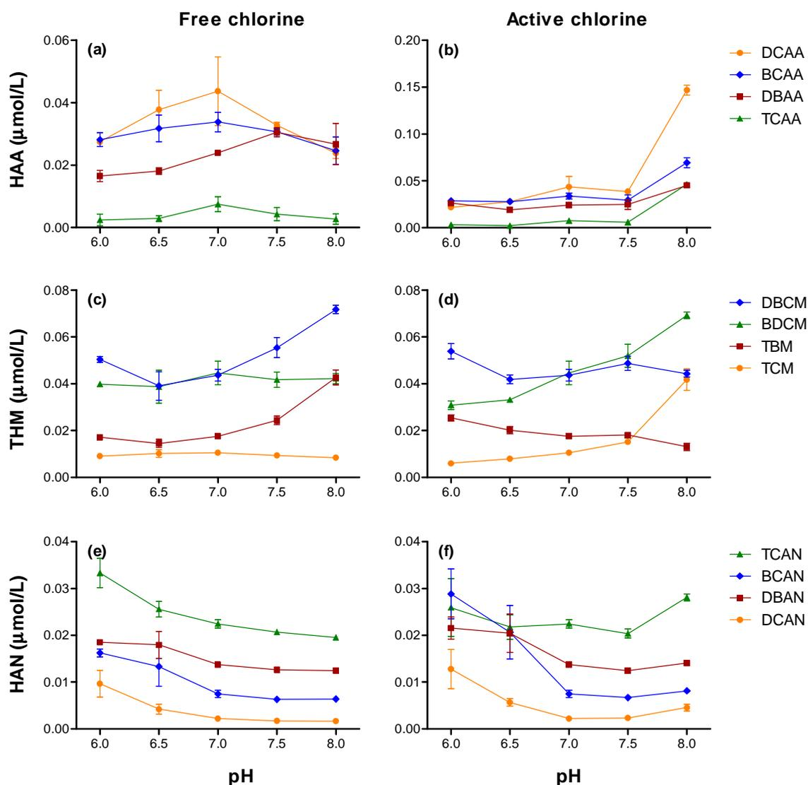
**Figure 3.** Effect of pH on THMs, HANs and HAAs formation from chlorination of BFA with constant initial concentration of free chlorine (a, c, e) and active chlorine (b, d, f), in the presence of bromide (1 mg/L). The error bars represent the standard deviation of three replicates. (Reaction time = 48 h, temperature = 25 °C and BFA addition = 1 mg TOC/L). Abbreviation of compounds is found in Table 1.
