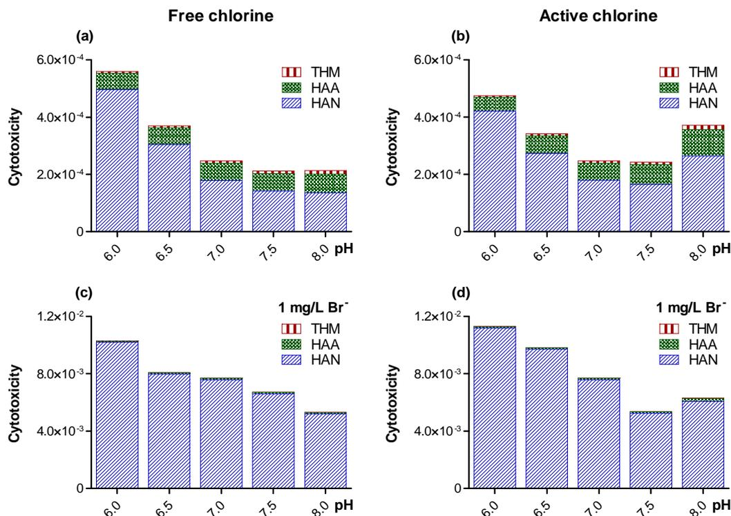
**Figure 5.** Estimated cytotoxicity of chlorinated BFA solution with constant initial concentration of free (a,c) and active chlorine (b, d), at  $6.0 \leq \text{pH} \leq 8.0$  in the presence and absence of  $1 \text{ mg/L Br}^-$ .
