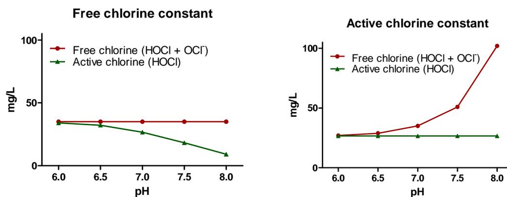
**Figure S1.** The initial concentration of free and active chlorine in the two chlorination approach: constant initial concentration of free chlorine (left) and constant initial concentration of active chlorine (right).
