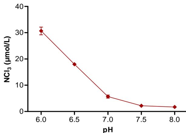
**Figure 4.** Effect of pH on NCl<sub>3</sub> formation from chlorination of BFA at constant initial concentration of free chlorine. The error bars represent the standard deviation of treatment duplicates. (Reaction time = 24 h, temperature = 25 °C and BFA addition = 1 mg TOC/L).
